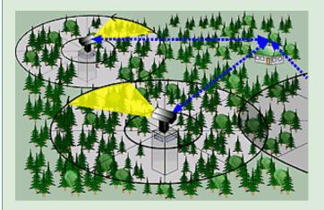
Figure Automated Forest Fire Monitoring System "Fire Watch". Sectors and images are shown on a monitor; the detected fire location is identified on a topographical map. (Source: IQ wireless Ltd)
